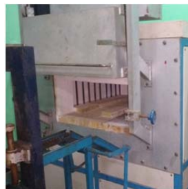
Figure 1(a). Closed Chamber Type Furnace
